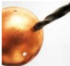
A quick way to remove the burr is to grab a drill that's two or three times larger than your hole. Simply twist it in the hole to cut off the burr. I usually do this twisting by hand, but if you have many holes to do, it's easier on your fingers to put the drill into a holder like a pin vice.
